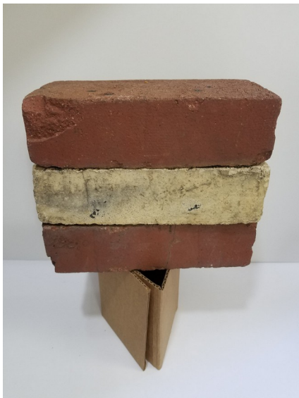
Figure 1: The corrugations shown here run vertically. They can support a LOT of weight!
