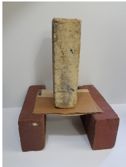
Figure 2: The corrugations shown here run from brick to brick. In this way, they have excellent bridging strength.
